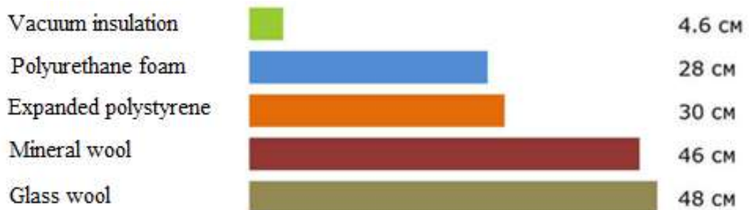
Figure 5 - Comparison of the thermal performance of vacuum insulation with other thermal insulation materials.
